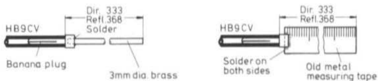
Fig. 15: The two different outer parts of the elements
