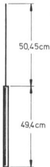
Fig. 5: Dimensions and construction of the vertical element
