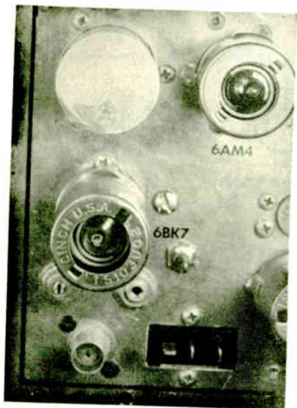
PHOTO 2. Top view of mixer cavity shows position of hole for coupling link and of capacitor C11 (right of tube).
