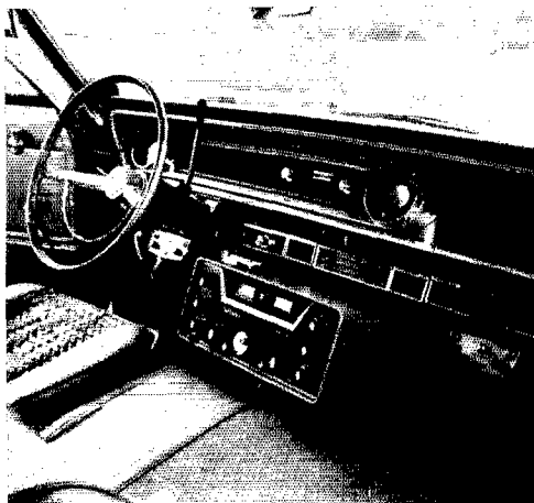
Most fm mobile work is done with trunk-mounted equipment. This means that only the control head, speaker, and tone-signaling box (if used) are mounted in the driver's compartment. In this view of the W6TEE mobile installation one can see the fm controls, plus an hf transceiver for use on other amateur bands.
