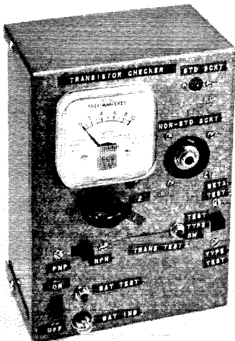
Front view of the transistor checker. The phone jack, which is used with a three-conductor plug and clip leads to make contact with transistors that don't have wire leads, is insulated by a piece of Plexiglas from the metal cabinet.
