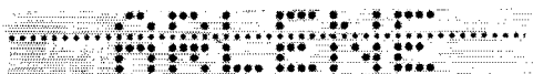
Fig. 3—Punching the actual characters of the alphabet can be done by using a code such as the one given in Table I.
