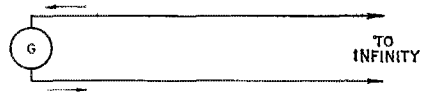
Fig. 1—An imaginary two-conductor line extending to infinity. Arrows show that the current in one wire flows in the opposite direction to current in the other; this relationship is true throughout the entire length of the line, although the actual currents periodically reverse direction as the polarity of the generator's voltage reverses each half cycle.
