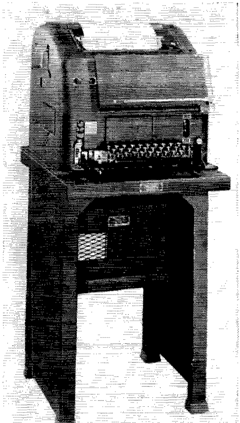
The Model 15 page printer with table. This type of machine is in use in a great many amateur RITTY stations.
