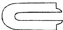
Fig. 2—100-230-Mc. inductor. The drawing is full size and may be used as a template.
