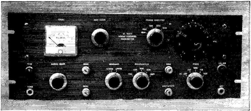
A phasing-type s.s.b. exciter. All adjustments can be made from the 7-inch rack panel. Controls along the top, from left to right, are for antenna coupling, the multiband tuner in the final, and the v.f.o. Along the bottom are connectors for microphone input and test-tone input (for alignment purposes), audio gain control, carrier null controls, sideband selector, band switch, excitation and final grid-tuning controls, mode switch and key jack. (Photos by Rogers H. Connell, WFLA-TV News-Photo.)
