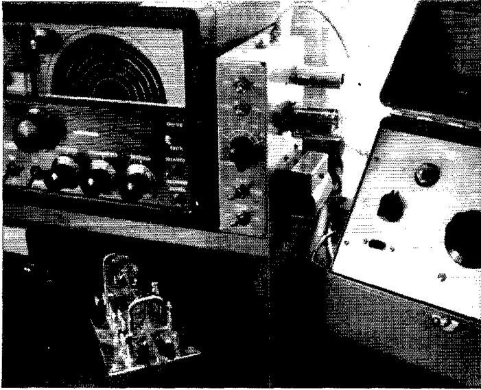
Monitrol mounts handily alongside the station receiver. From top to bottom the switches are, as designated in Fig. 1, S 5 , S 4 , S 1 , S 3 and S 2 . Conelrad monitor can be seen at right.
