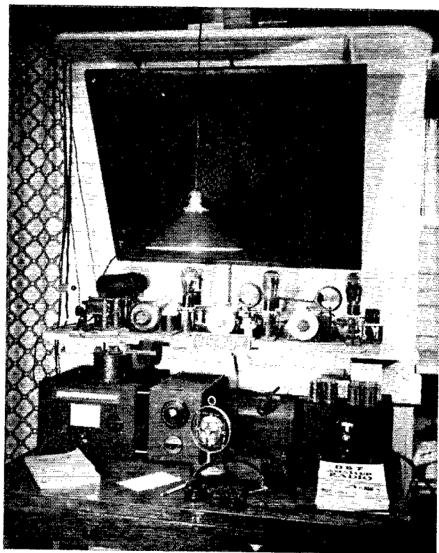
Here we have a mock setup of the early 1930s. Across the table, from left to right, are an FBX receiver, a pre-selector, a power supply, and an SW-3 receiver. The shelf above holds a crystal-controlled transmitter using a pair of 210s in the final. Those were the days!
