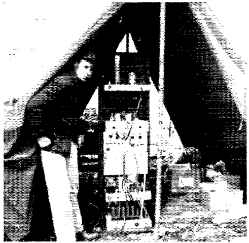
Top single-operator station in June V.H.F. Party was W1UIZ/1, Mt. Equinox, Vt. Shown here with rear view of the rack-mounted gear for 50, 144, 220 and 420 Mc. is maintenance engineer, W1WID.
