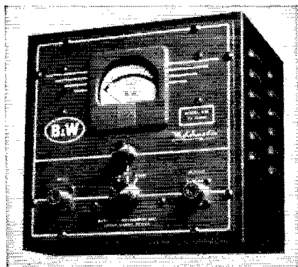
The "Matchmaster" is a combination of dummy antenna, r.f. wattmeter, and s.w.r. bridge, and is useful for testing and adjustment of transmitters and antenna systems. Dimensions are 8\frac{1}{4} by 8\frac{1}{4} by 6\frac{1}{4} inches.
