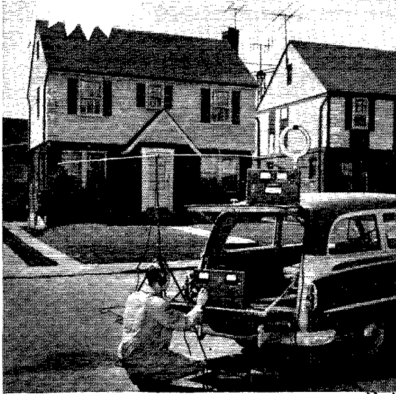
Actual measurement of radiation using RCA field intensity equipment. Note close proximity of TV antennas without TVI.
