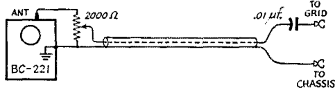
Fig. 4—Using the BC-221 frequency meter as a signal generator for filter and i.f. alignment. If a 221 is not available, any oscillator covering the necessary frequency range with adequate handsread may be used, as described in the text.
