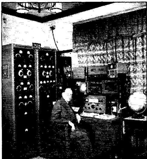
The well-engineered installation at ZS6Q, Johannesburg, operated by Harry Chemik. The gear features such items as a BC-221 VFO with slug-retuned exciter, separate finals for four bands, and rigidly-monitored modulation. Antennae include close-spaced and Lazy H beams plus 40- and 80-meter folded dipoles.
