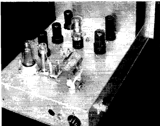
A rear view of the exciter. The 6SN7 and the Millisee relay (in metal tube envelope) to the right of the VR tube are used in the keying circuit. The linear condenser standing alongside the 2E26 furnishes a short return path for harmonics.
