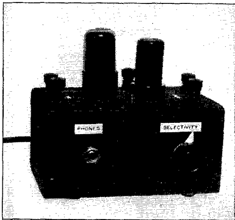
This little audio amplifier has amazing selectivity, derived from a negative-feed-back circuit working through a twin-“T” network. The simple circuit requires only three triodes and a few resistors and condensers.
