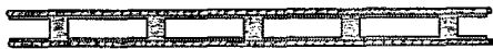
Fig. 4 — Method of "weatherproofing" feedlines made of Twin-Lead. Some of the dielectric is removed, leaving only enough to maintain line spacing.
