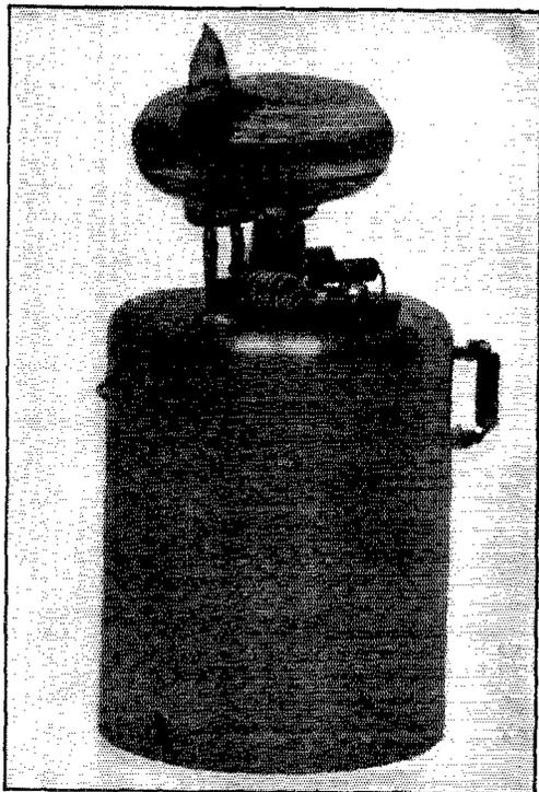
The oscillator assembly with the 703A in place. The grid leak,  $R_g$ , is at the right.
