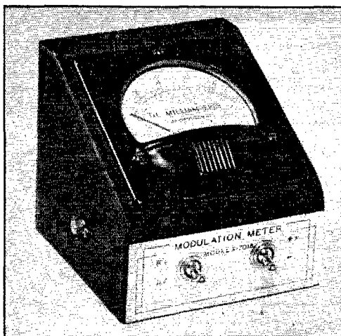
A simple direct-reading modulation meter. The scale of the 1-ma. meter reads directly in percentage of modulation. The screwdriver adjustment on the side is for setting the r.f. level.
