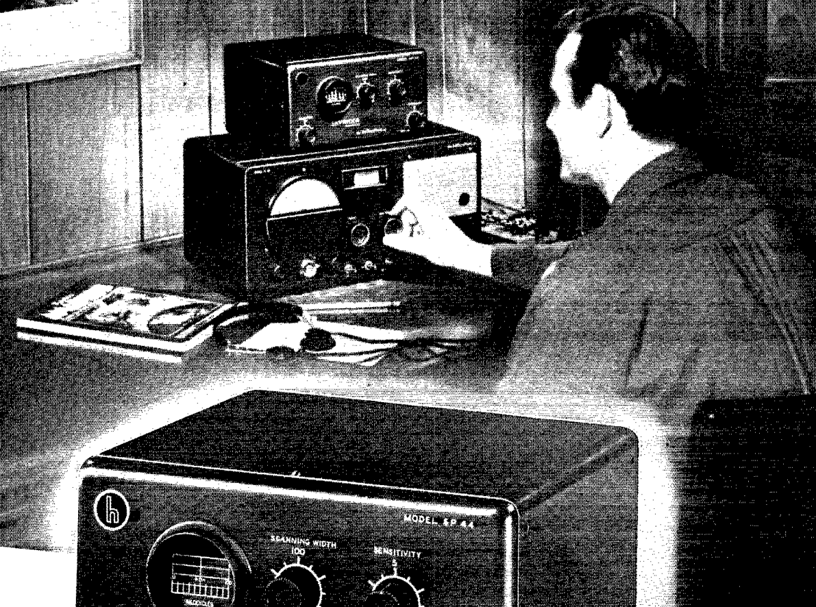
Photo above shows Hallicrafters SP-44 Panoramic in use with Hallicrafters receiver, the Model S-40.
