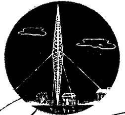
1930 Half-wave vertical radiator, now in general use, was developed into practical form. It greatly improved signal output of broadcast stations.
