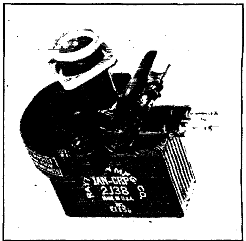
The 2J38 is a "compact" lower-powered magnetron of the package type that was used extensively in aircraft radar. The output fitting is for coaxial line.
