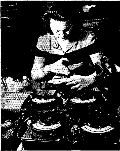
From this girl's skilled fingers, sensitive precision meters receive delicate final adjustments at Westinghouse.
