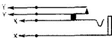
Fig. 1 — Diagram showing connections to filament-lighting jack. Terminals marked "X" go to the headphone circuit, while those marked "Y" are connected in series with one side of the filament.
