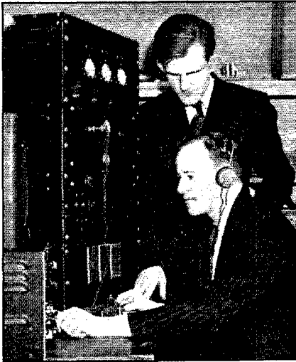
Leo Sadowsky, W2OFU, deaf, dumb and blind radio amateur (seated) and his instructor, Robert Gunderson, W2JIO, also blind. Leo "hears" through the sensation produced by 60-cycle a.c. in the 'phones, keyed by a relay in the receiver output.
