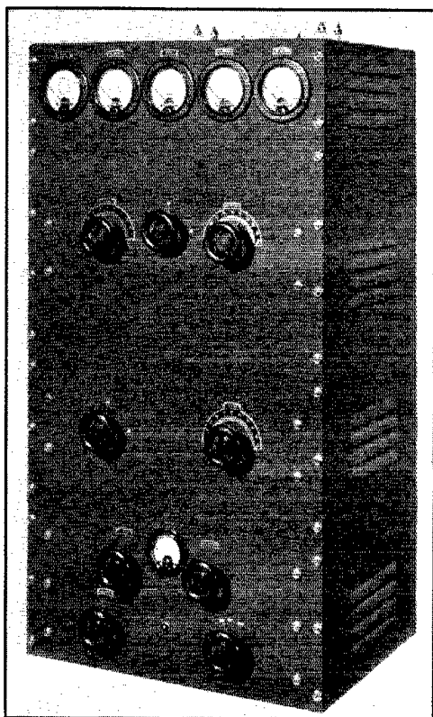
THE TRANSMITTER IS A 60-80 WATT C.W.-PHONE JOB
