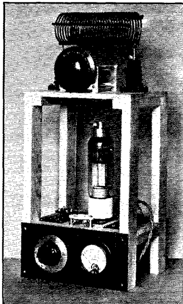
THE NEW RK-28 PENTODE IN AN EXPERIMENTAL TEST SET-UP
