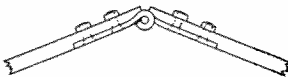
FIG. 1.—ONE METHOD OF HINGING SO THAT THE POLAR AXIS WILL BE AT THE SURFACE OF THE TWO PIECES BEING JOINED TOGETHER
