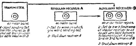
FIG 3—SETTING THE TRANSMITTER ON A "HOLE IN THE INTERFERENCE" WHICH WAS LOCATED BY MEANS OF THE RECEIVER A.
