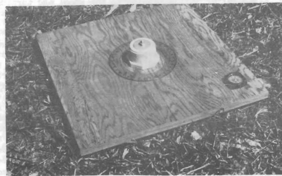
Fig. 7. Base, PVC plug, 360° setting circle; compass at right.
