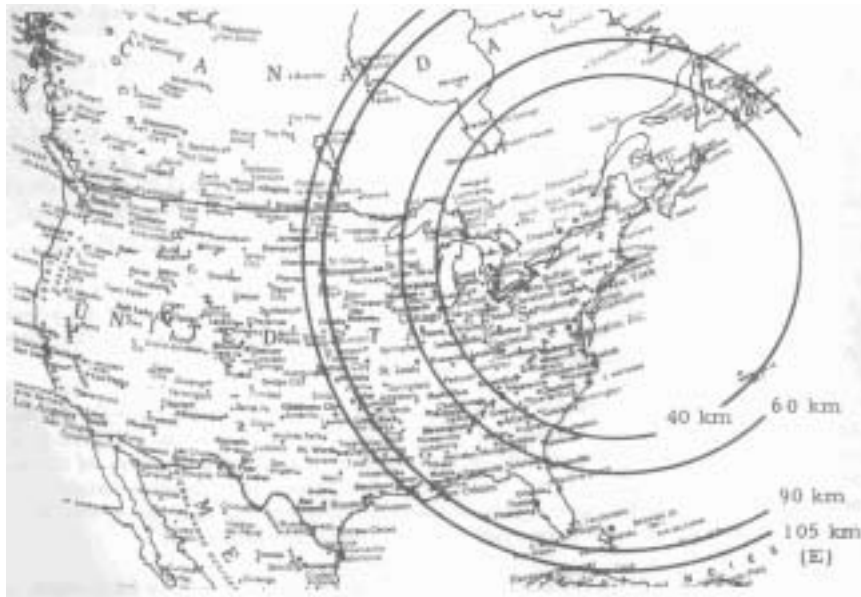
Figure 7. Maximum midday single D skip distances for different reflection heights. Chicago, Detroit, Cincinnati, and closer locations are audible; St. Paul, Memphis, and beyond are not. (From Greater Boston)
