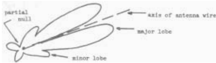
FIGURE G: Effects of Ground Plane on Vertical Pattern
