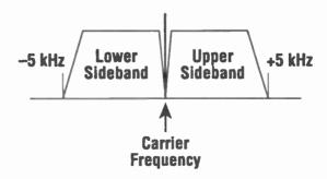
Figure 1. Normal Double-Sideband Spectrum
