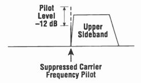
Figure 2. Normal Broadcast SSB Spectrum
