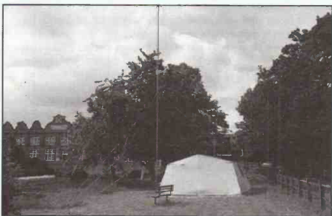
You don't need a big aerial on Field Day. Gravesend RS G3GRS/P have had great success with an 82m centre fed on an 11m mast, with one end of the aerial across a river.
