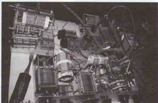
'Open plan' ATU system - six separate ATUs allow instant band change
