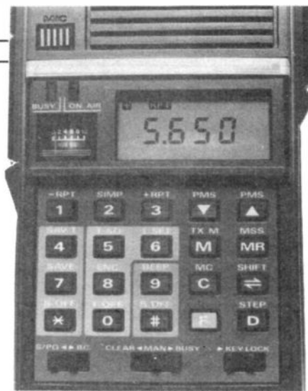
The keypad of the FT209R and RH are identical bar the name on the front.
