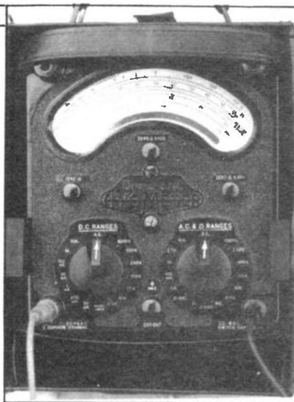
The Model 8 Avometer, a high quality, general purpose, analogue multimeter.
