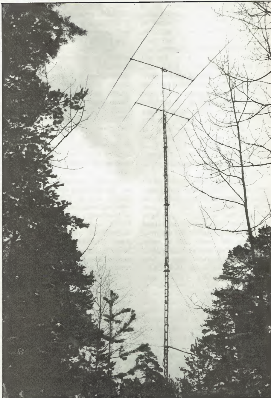
Club station SLOZG is almost bound to be participating in the WPX contest at the end of March. Their big signal comes from these antennas: 2 elements on 40m and 4 elements on 10m. There is another tower supporting antennas for 15, 20 and 80m.
