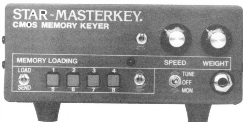
Fig.1 Front panel of the keyer, with toggle switches set prior to clearing memories.
