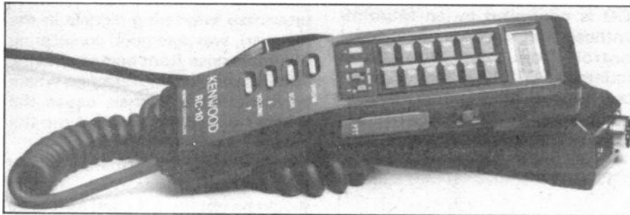
The optional RC-10 handset will allow remote control and cross-band duplex working.
