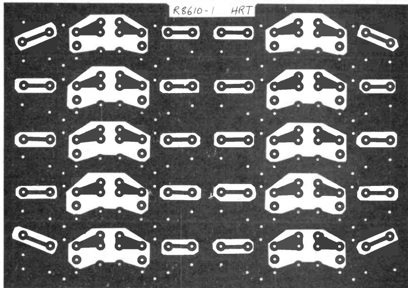
Fig. 8 Foil pattern for the filter PCB.
