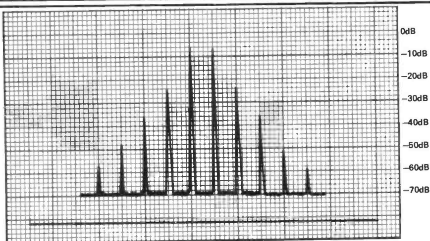
IC505 two tone transmitter IMD test again at high power setting.
