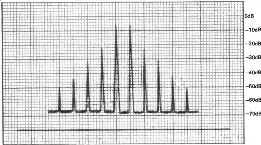
FT690R two tone transmitter intermodulation deviation at high power setting.
