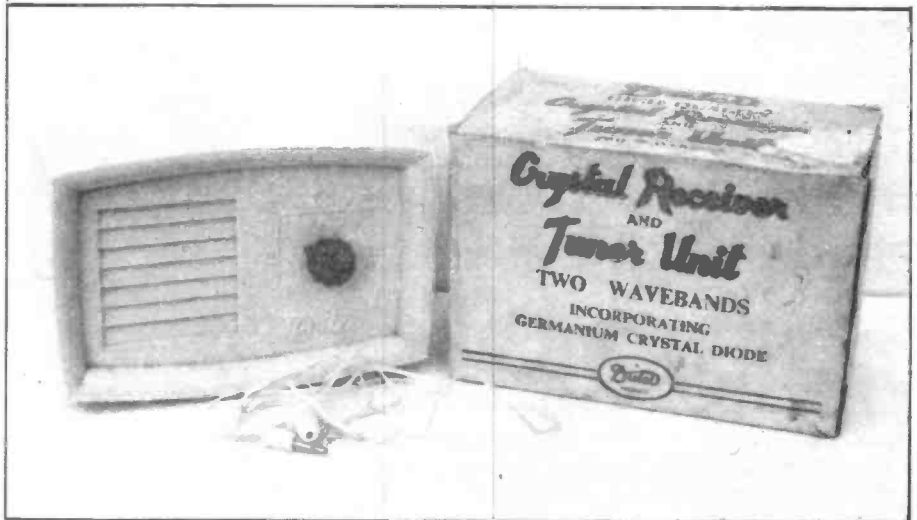
Radio comes full circle with a 1950's germanium crystal diode set in a plastic case.
