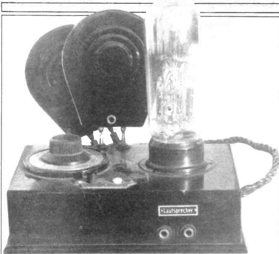
Receiver made by Loewe RC of Germany circa 1928 with three triode valves in one – so much for integrated circuits!!
