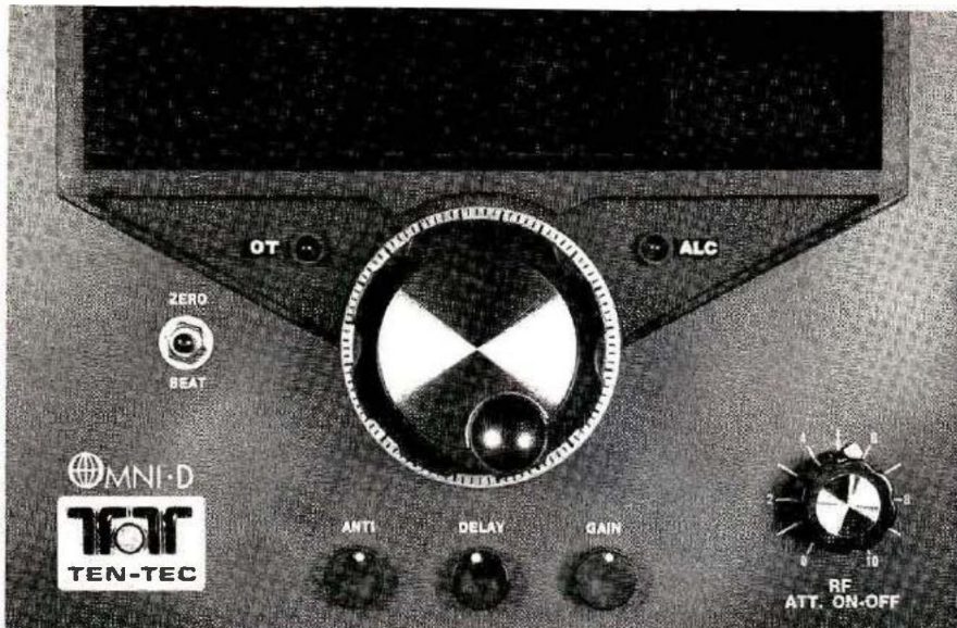
Fig. 11. Voice-operated transmit (VOX) controls make the operator's life easier. All you need do is speak, and electronic wizardry does the rest. The controls shown here, below the main tuning knob, are for adjusting the sensitivity and time-delay of the VOX; the one labeled "ANTI" is to prevent your own speaker from turning the rig on.
