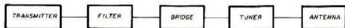
Fig. 2. The tuner should be connected between your transmitter (or transceiver) and the transmission line to the antenna. If you use a filter (highly advisable), it goes immediately after your transmitter. You will need an SWR meter to adjust the tuner, so if you already have one, you do not need to build it into this project.
