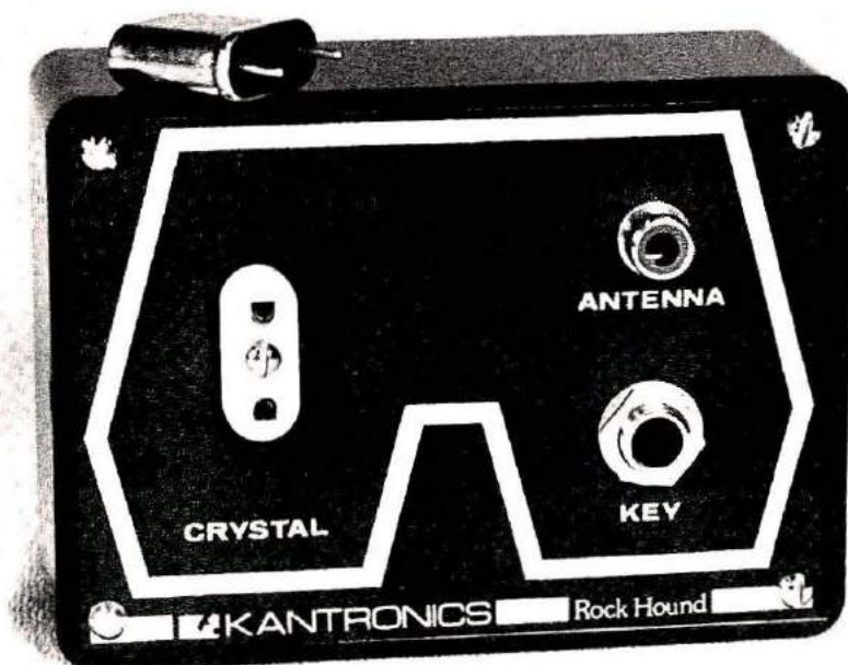
The Kantronics "Rock Hound" is a small transmitter which runs on 12 Vdc.
