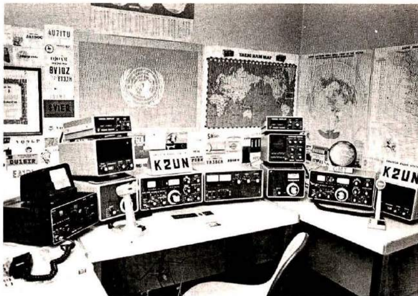
The United Nations amateur radio station, K2UN, features a highly functional equipment arrangement. Completely furnished by Yaesu Electronics, the console includes dual high-frequency transceivers and a separate 2-meter station. All equipment can be reached by the operator from a single operating position (photo courtesy Yaesu Electronics).
