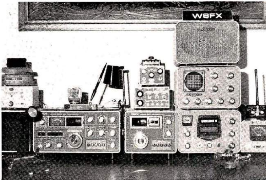
A partial view of the author's station showing equipment arrangement. When stacking pieces of equipment on top of each other, consider off-on duty cycle. If equipment runs continuously, make sure sufficient air space is available between the stacked pieces to provide ventilation.
