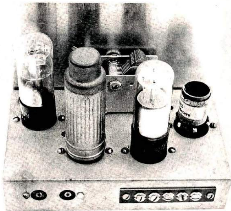
Doerle type regenerative receiver built from a 1938 kit. This battery-operated receiver uses a 1F4G as a detector, a 1H5G audio amplifier, and a 1C5G second audio stage. The 1F4G detector is in the center with a metal shield over the tube. Shortwave spectrum from 10 to 200 meters is covered with four plug-in coils. When wired up, the receiver worked right off the bat!
