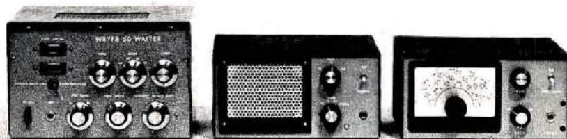
Amateur Radio equipment does not have to be fancy, nor does it need to cost a lot. In addition to buying used equipment, and building kits, you can make your own transmitters and receivers, as shown here. The unit at the left is a 50-watt transmitter, described in a three-part series that started in July, 1978; the two smaller units are a receiver and the power supply/converter for it, from the February, March, and April, 1979, issues of Ham Radio Horizons .
