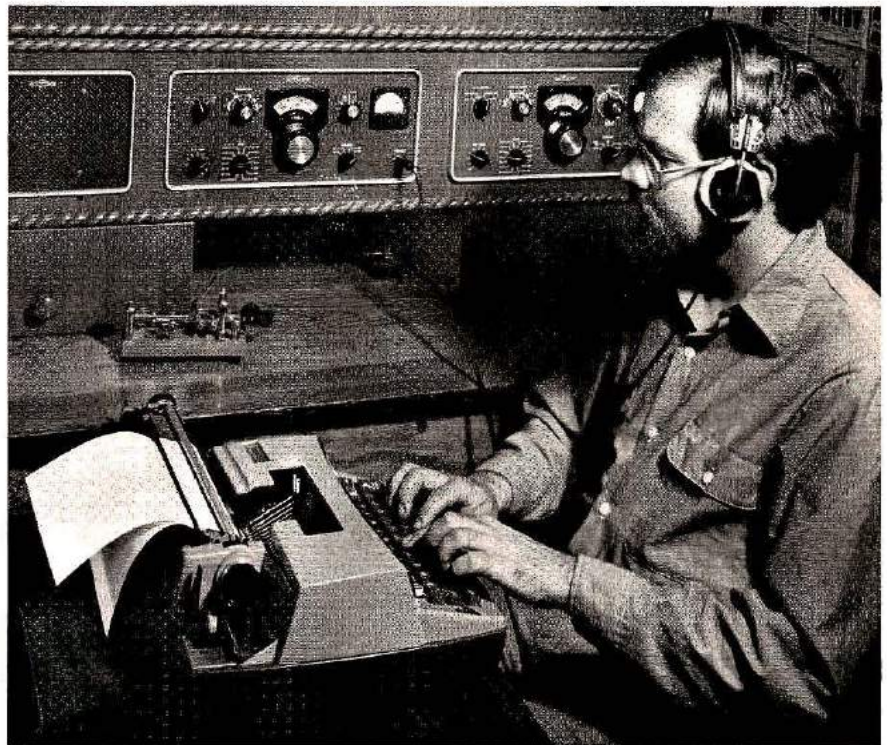
CW lends itself to simple and efficient station layout. In the tradition of the old-timers, the author copies high-speed CW on a typewriter, or "mill." With practice, typewritten copy becomes both easy and automatic. The semi-automatic key, or "bug" is used most of the time, but a traditional straight key lurks in the console niche ready for a quick shift to slower speeds for excursions in the Novice bands.
