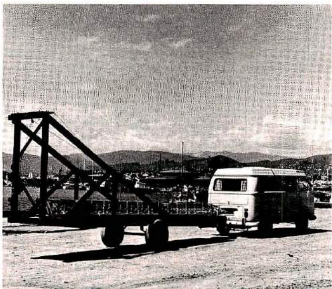
A wooden tower trailer — or is it a guillotine? This is the prototype trailer, forerunner of the others described. Here it is shown with a small tribander, although it has been used with arrays as large as a 5-element 15-meter beam, which it will support at 70 feet. Note the diagonal braces from the wooden uprights shown at the right. They contact the ground to provide increased stability for the tower. A cable and turnbuckle between the legs provide tension to keep them firmly in contact with the ground.
