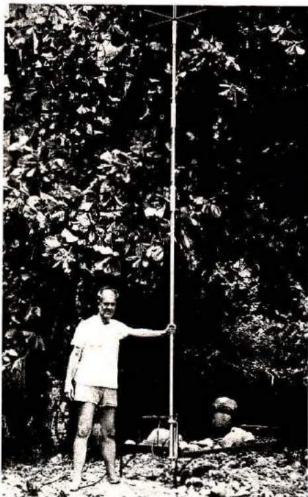
Author TI9AEL and the vertical antenna, which had been mounted on the frame of an old army cot salvaged from the beach.
