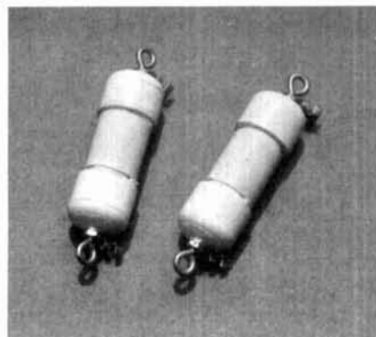
Commercial loading coils.
