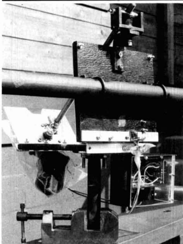
Left front view of elevation drive at maximum elevation showing fiberglass rod support for antenna. Also shown is electronics box with limited switch control circuit.
