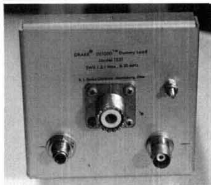
End panel showing the coaxial connector plus added RCA phono and BNC jacks.
