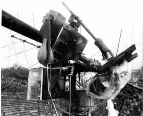
Left rear side view of antenna drive system. Elevation pot arm with lead weights is visible at top.
