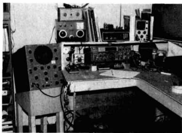
fig. 2. Two recurrent-sweep scopes are used; larger to monitor receiver i-f, smaller as RTTY tuning indicator.
