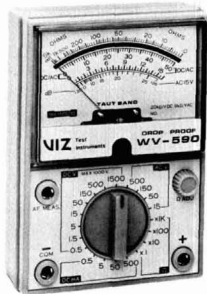
fig. 1. The oldest form of multimeters — the VOM.
