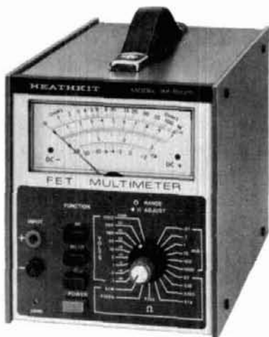
fig. 2. High input impedance is — provided by the FET multimeter.
