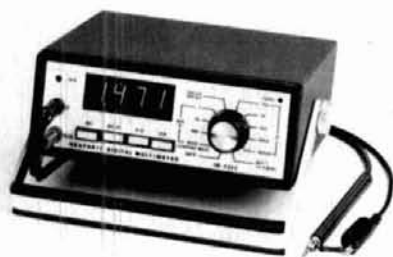
fig. 3. Bench-type digital multimeter.
