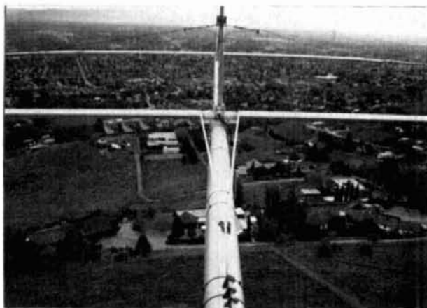
fig. 1. Sighting along boom of a KLM 4 element Yagi reveals unobstructed near field topography.
