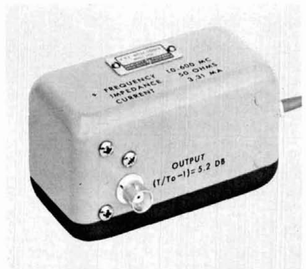
The Hewlett-Packard model 343A VHF Noise Source utilizes a temperature-limited diode, and can be used from 10 to 600 MHz (courtesy Hewlett-Packard Company).
