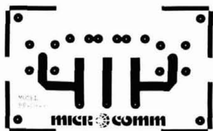
fig. 2. Full-size printed-circuit layout for the three-pole 1296-MHz bandpass filter. Etched on double-clad 1/16" (1.5 mm) fiberglass-epoxy circuit board; the unetched side serves as a ground plane.
