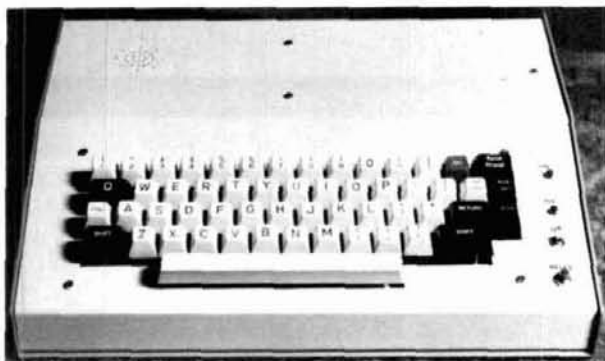
The CW keyboard is housed in a 14 x 11 x 3 inch (36x28x8 cm) cabinet available from Nu Data Electronics, 104 North Emerson Street, Mount Prospect, Illinois 60056.
