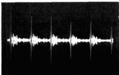
Fig. 2. SSB signal after processing with LSP-520BX. The once weak valleys are now strong peaks. Our NCX-3 now puts out 100 watts of average power.
