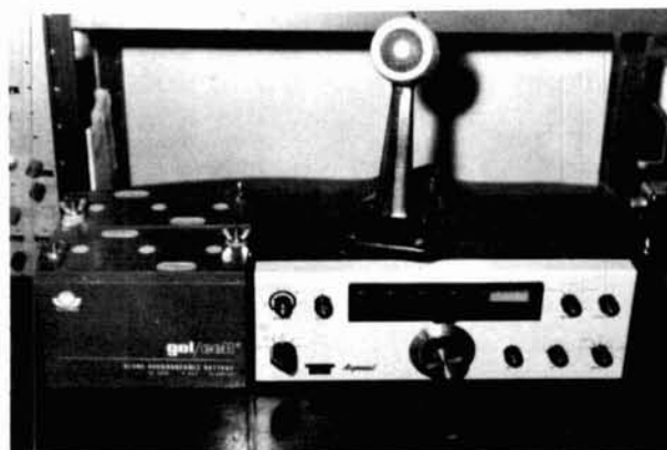
fig. 14. Ten-Tec transceiver installation with 6-volt Gel/Cel dry electrolyte batteries.
